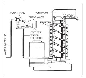
The ice, being costantly lifted up, meet the tooth of the ice breaker which is fitted on the top end of the auger, where it gets compacted, cracked and forced to change from vertical into horizontal motion to be discharged out, through the ice spout, into the storage bin.
