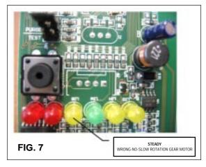
When the gear motor rotating speed is slowed below 1300 r.p.m. from the normal speed of 1400 r.p.m. the Electromagnetic Safety Device transmits an electrical signal to the MICROPROCESSOR to stop immediately the unit operations like it occures for the wrong rotation, with the lighting-up of the 3RD YELLOW WARNING LED. This to relieve from the excessive load all the electrical and mechanical components of the entire Drive System and extend their durability.
