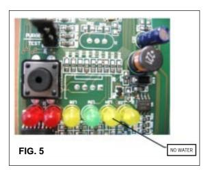
**NOTE**. The water level sensor detects the presence of sufficient water in the float reservoir and confirms it to the micro processor by maintaining a low voltage current flow between the two sensors using the water as conductor.
