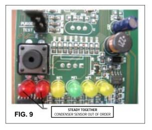
**NOTE.** To restart the unit after the shutoff caused by the hi condenser temperature, it is necessary to push the RE-SET button (after having remedied to the causes of unit stoppage) or to switch OFF and ON the power line main disconnect Switch.
