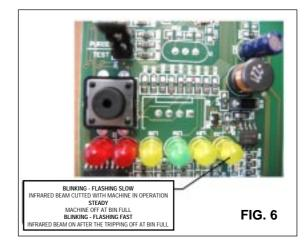
NOTE. The ICE LEVEL CONTROL (INFRA-RED SYSTEM) is independent of the temperature however, the reliability of its detection can be affected by dirt and scale sediment which may deposit directly on the light source and on the receiver.
